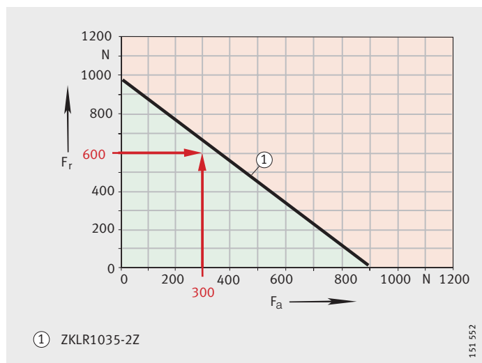
Figure 23 Static limiting load diagram – example ZKLR1035-2Z
