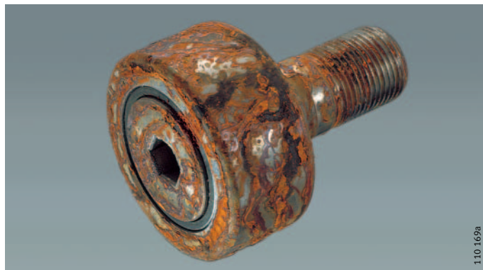
Figure 26 NUKR52 without plating after salt spray test
