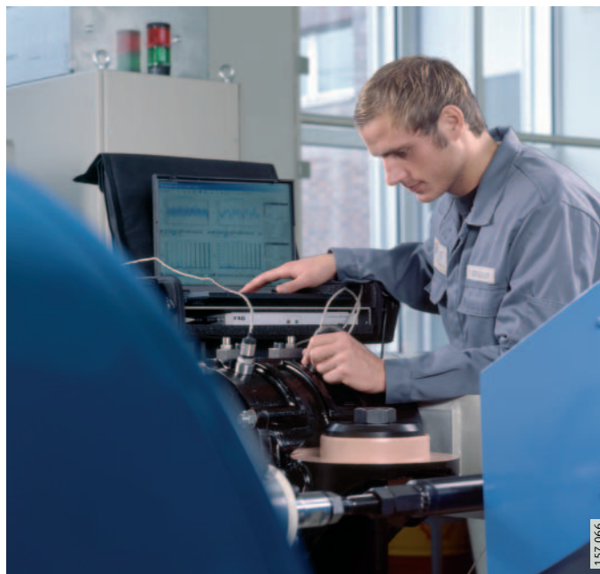
Figure 9 Condition-based rolling bearing monitoring using Bearing Analyser
