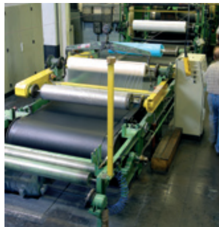
A three roll calendering machine shown with a processed width of cover fabric
